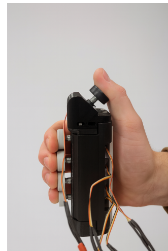
Fig. 1: Prototype of the modular grip-force measurement system developed in this thesis, shown here configured for the Medium Wrap grasp
