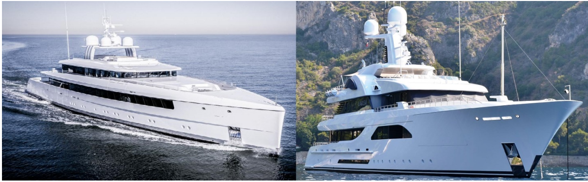
Figure 4.15: On the left the straight bow and on the right the flared bow[11, 14]
