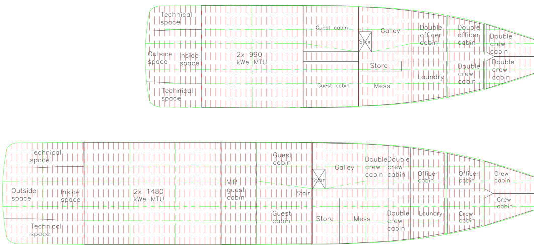
Figure 4.19: The construction overview of the main deck for the minimum and maximum length, in green the primary stiffeners and in red the secondary.
