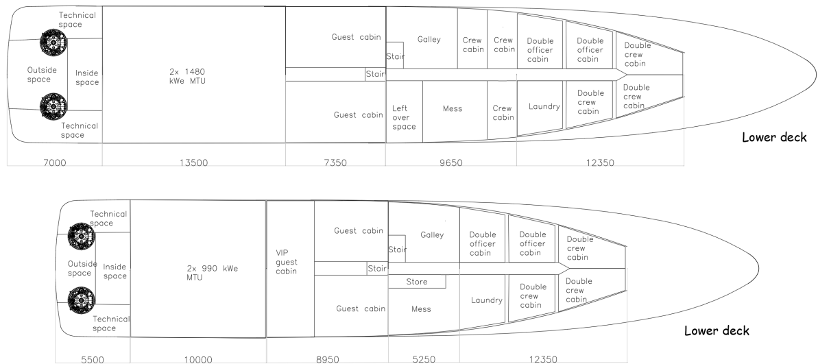
Figure 5.3: Two lower deck arrangements to illustrate the difference due to different compartment lengths
