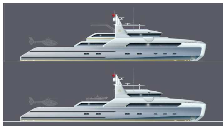
Figure 3.13: The ER yacht design concept of a yacht with module swapping capacity to change it from family yacht to an expedition yacht[3]
