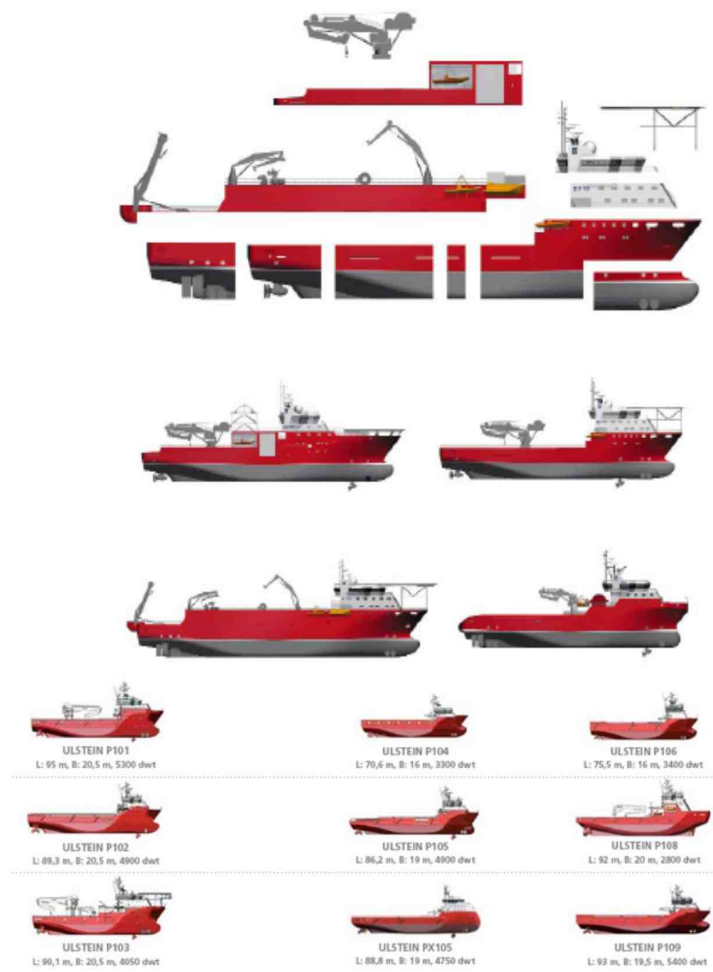
Figure 3.12: The modules and some variants of Ulstein's modular design approach[7]
