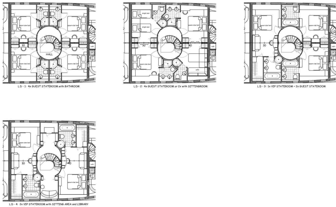
Figure 3.2: The four possible options for the SL39 lower deck guest cabins. The first option shows 4 identical rooms, the second option shows two normal staterooms and two staterooms that can be converted from a sitting room to a stateroom. The third option has one large VIP room and two normal staterooms. The last and fourth option features two VIP staterooms.[9]
