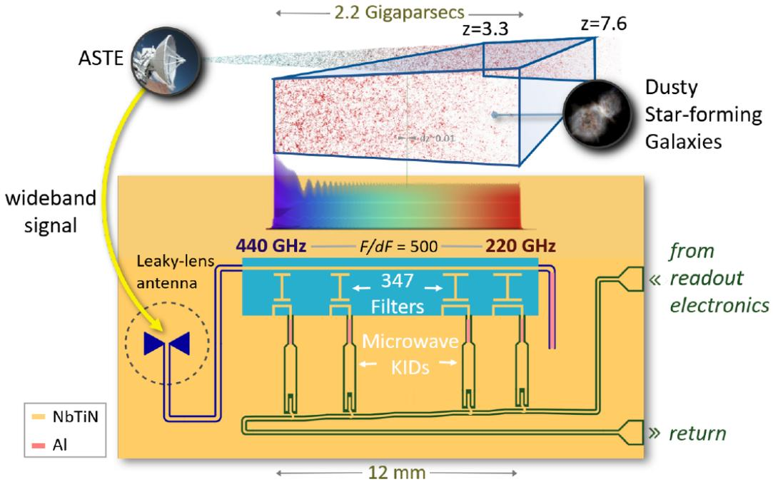
Figure 2.1: A schematic representation of the DESHIMA 2 chip. This image is taken from [7].
