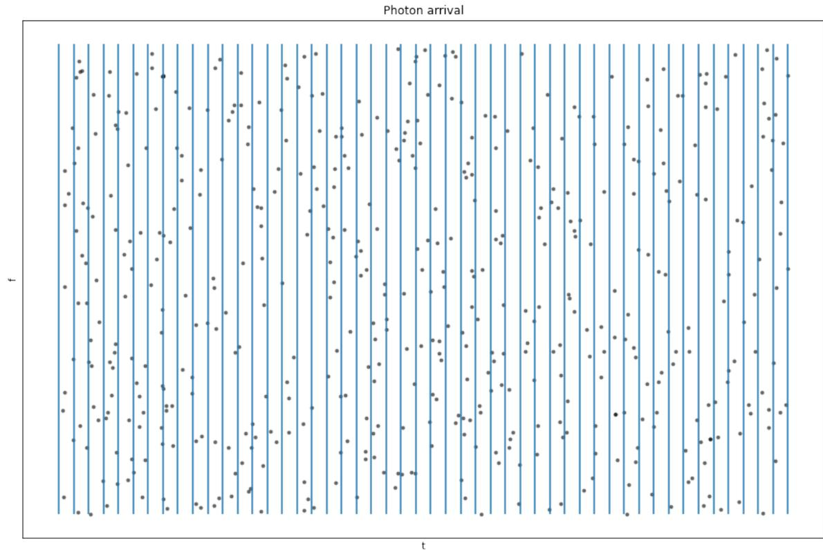
Figure 7.3: A representation of a the wide-band signal that is split into infinitesimally small bins. Photon number still conserved in theory.
