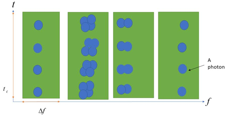
Figure 7.6: A representation of wide-band signal of non flat spectrum divided into 4 sub-bands
