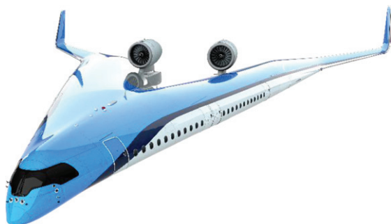
Fig. 1. The Flying V showing that passengers are located in the wing.
