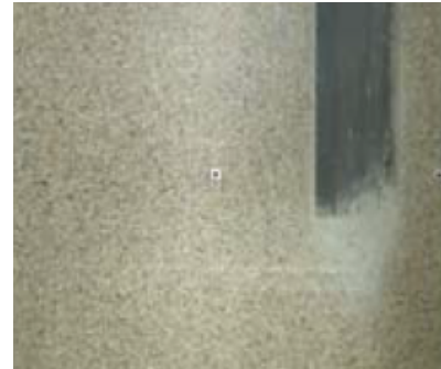
(b) "nose cone" of soil beneath pile tip
