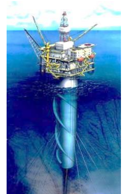
FIGURE 3-1 OFFSHORE SPAR STRUCTURE
