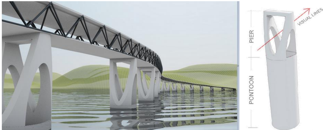
FIGURE 9-3 BRIDGE PIER AND PONTOON SHAPE (WITH RANDOM BRIDGE GIRDER LAYOUT) [38]
