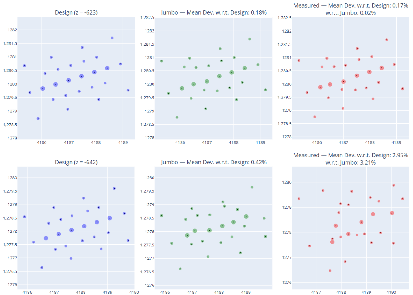
Figure 19: Opening slot plan views, collar and toe level.
