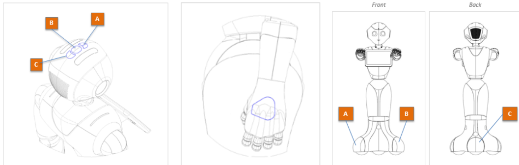
Figure 3.4: Tactile sensors in the head (left), hands (center) and bumpers (right) [22].
