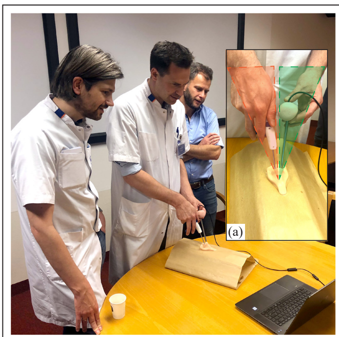
Fig. 48: Three participants testing the NeuroPunch. Close-up (a) depicts the hand positioning when using the NeuroPunch, in which the interaction between the endoscope and NeuroPunch is clearly visible.
