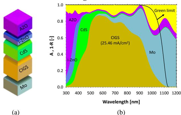
Fig. 1: a) Simulated model. Thicknesses of the layers from bottom to top (in nm): 200, 500, 70, 60 and 230. b) Simulated absorptance and reflectance (yellow) compared to Green absorption limit (solid black line) for a 500-nm CIGS layer.
