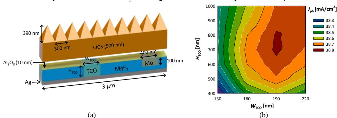
Fig. 3: a) Rendering of the back contacted CIGS solar cell and b) implied photocurrent density as a function of height and width of n-contact.
