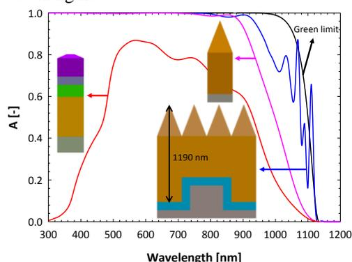
Fig. 2: Absorption spectra of the reference cell with a 500-nm thick absorber (red), a CIGS slab endowed with high aspect ratio pyramids and silver back reflector (pink), the same, but with the addition of diffraction gratings and a dielectric spacer at the back side (blue) and the Green absorption limit for a 1190-nm thick CIGS slab.
