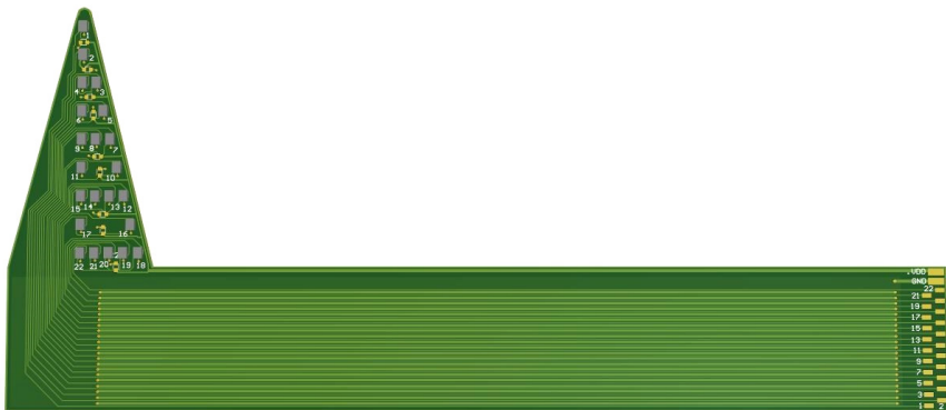
Figure 3.9: PCB manufactured with 22 MEMS sensors to be mounted on the surface of a serrated trailing edge. The image shows the backside of the PCB with the sensors installed.
