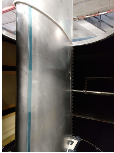
Figure 4.7: BANC NACA 63 3 -018 2D wing model mounted inside the Kevlar test section of the LTT wind tunnel.
