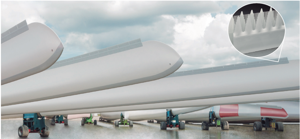
Figure 1.3: Wind turbine blades retrofitted with trailing-edge serrations. Adapted from [9].
