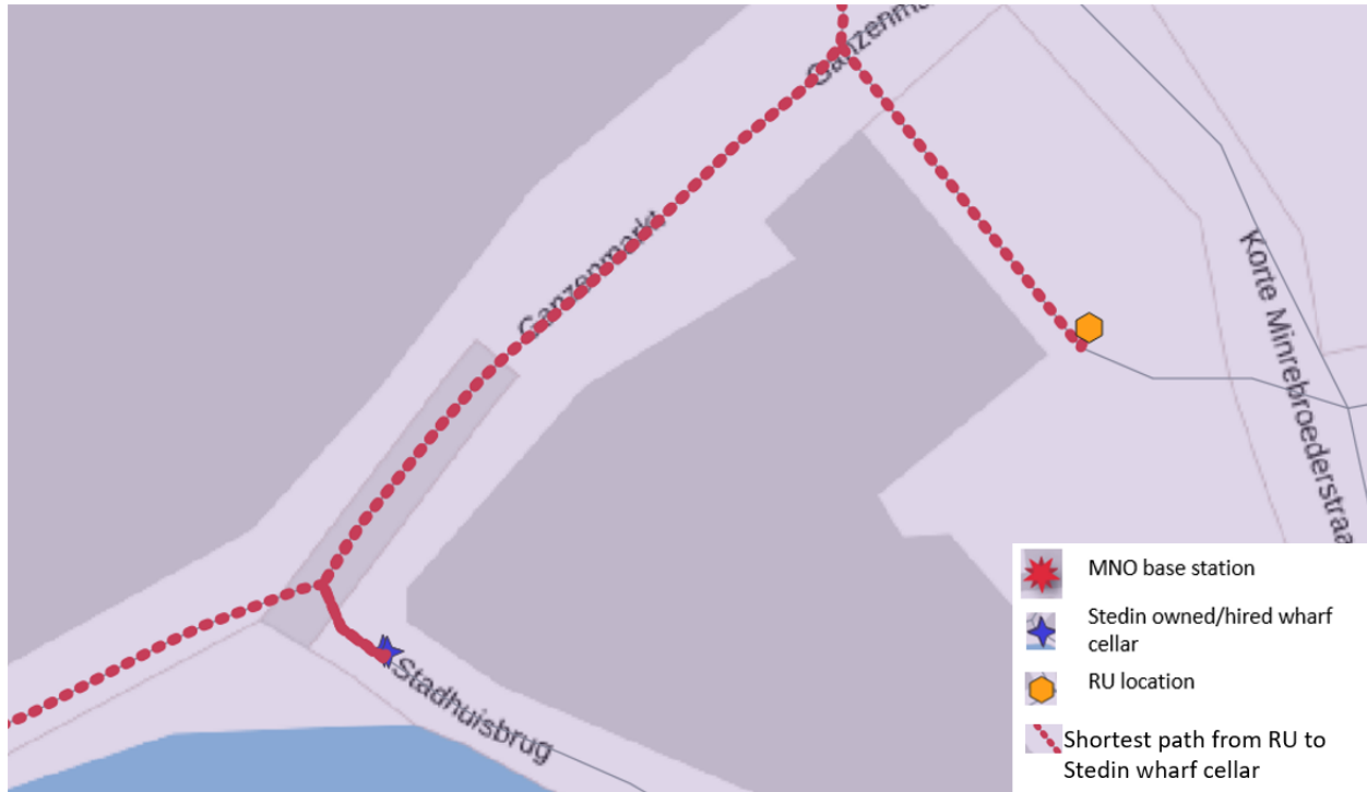
Figure 27: Shortest path from a RU to Stedin-owned/hired wharf cellar
