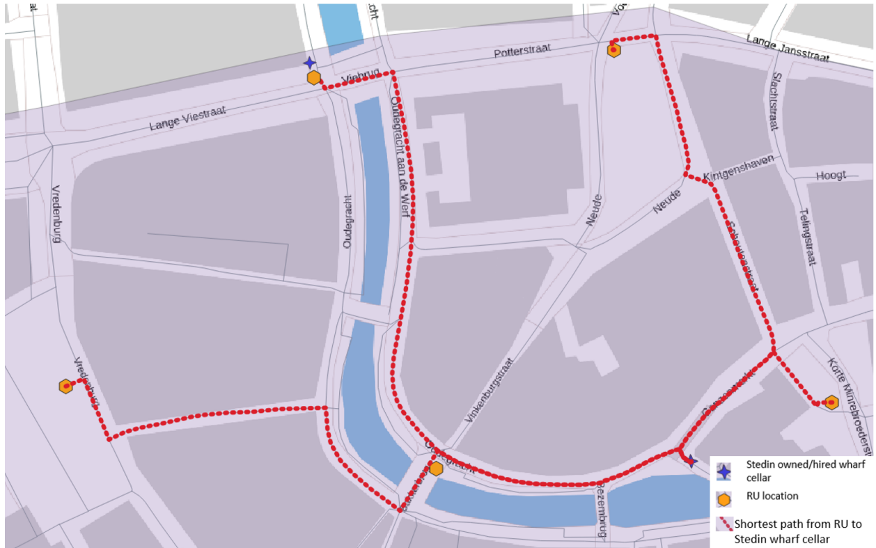
Figure 36: Five RUs connected to DU and CU located in the Stedin-owned/hired wharf cellar
