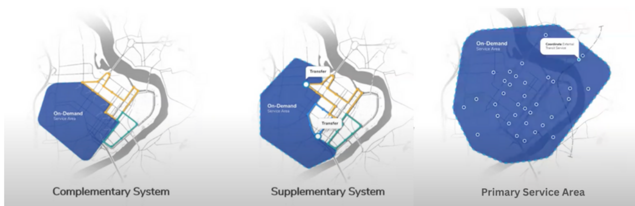
Figure 14. Three implementation frameworks in which DRT can support fixed route services. Credits: Klumpenhauer, et al., 2020.
