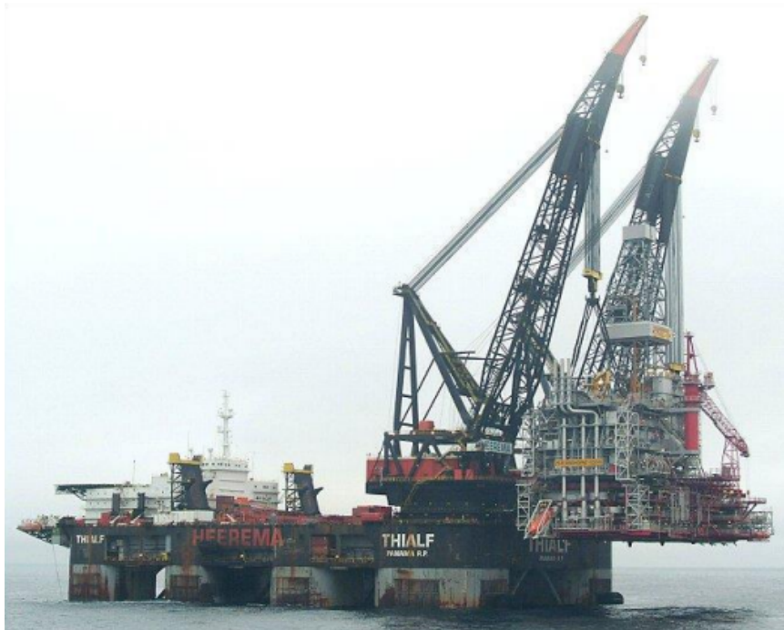
Figure 2.3: Heavy lifting crane vessel Thialf(Kaminski, 2012b)
