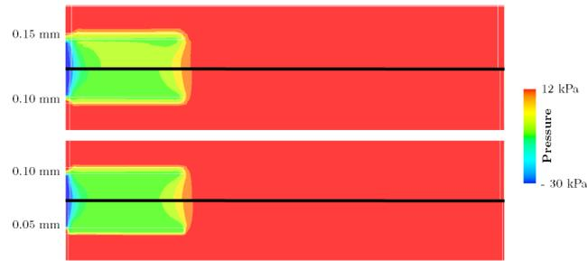
Figure 2.12: The pressure distributions of the 0.05 mm, 0.10 mm and 0.15 mm meshes compared at  $t=250$  ms. The upper halves of the velocity profiles are placed side by side, with the one half mirrored in order to evaluate the velocity profile more easily.
