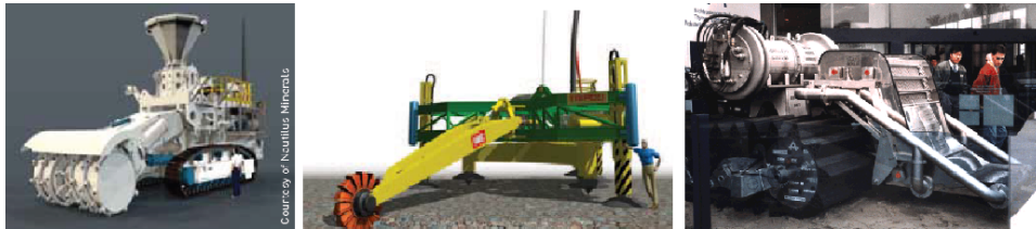
Figure 2.8: Drum cutter (SMD), auxiliary cutter (IHC) and nodule collector (IKS)
