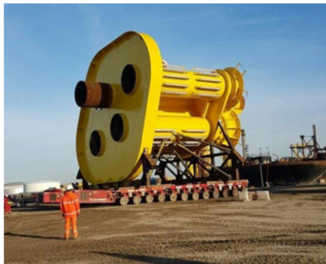
Figure 2.5: Mammoet SPMT carrying a jacket part for Maersk Culzean jacket at Vlissingen yard. Source: www.hfg.heerema.com
