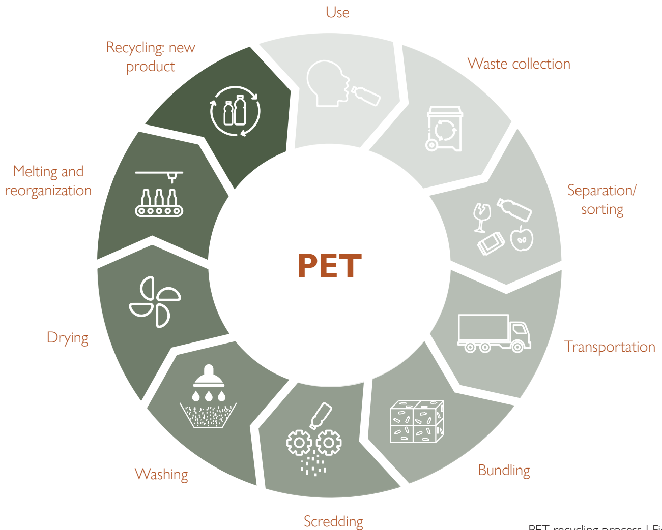
PET recycling process | Fig. 16
