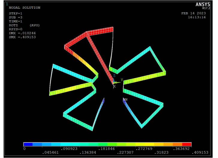
Fig. 11: FEM analysis of the deflection of the flexure mechanism at a torque of 200 \mu\text{Nm} .
