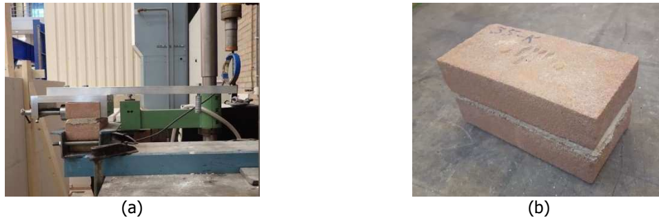
Figure 47 – Bond wrench tests: (a) improved set-up; (b) couplet specimen.
