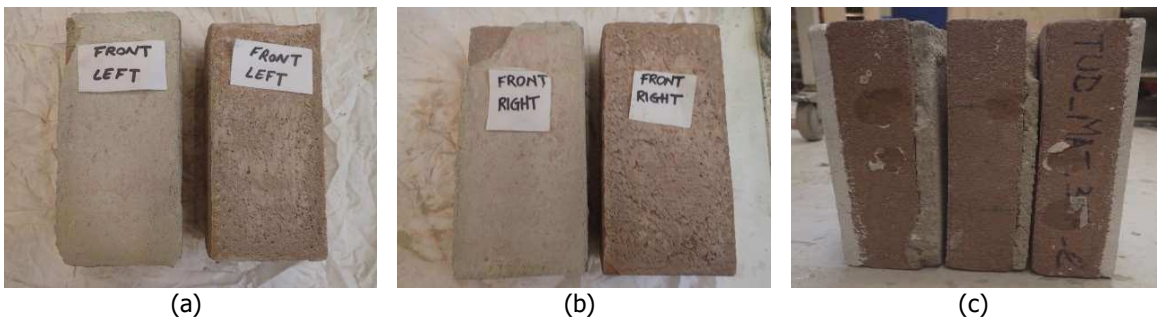
Figure 60 – Crack pattern of standard triplet under shear test: (a) front-left joint; (b) front-right joint; (c) front view.
