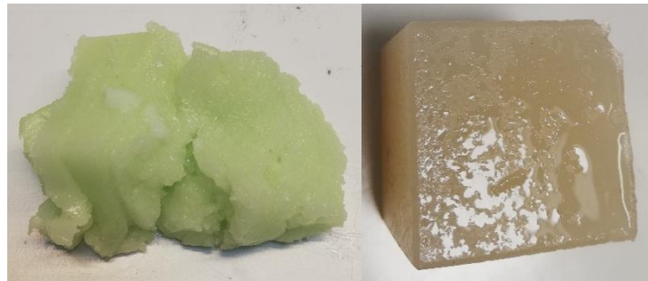
Figure 33: Agar-based phantom tissues with oil as additive. Left: oil with surfactant, right: oil
