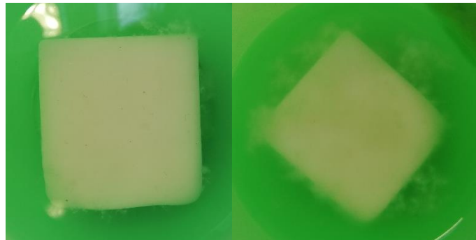
Figure 14: Gellan gum phantom stored in saline solution where phantom material gets loose. Left: storage for 2 weeks, right: storage for 3 weeks
