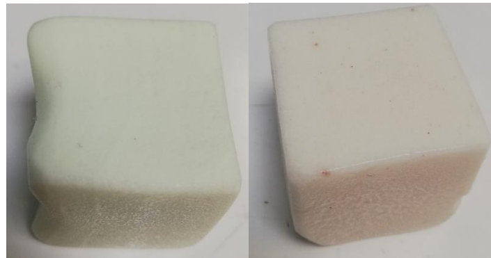
Figure 24: Gellan gum phantoms, left: oil as additive, right: PVC as additive
