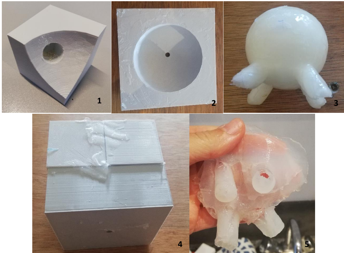
Figure 56: 3D printed sphere shaped mould. (1) One of the four smaller outer moulds to slide over one of the four cylinders of the inner mould. (2) The big outer mould. (3) The PVA-printed inner core. (4) The resulted 3D printed mould. (5) The failed sphere shaped cardiac phantom
