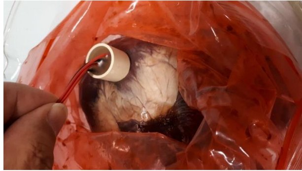
Figure 40: Measurements on porcine heart tissue with 4-points needle electrode
