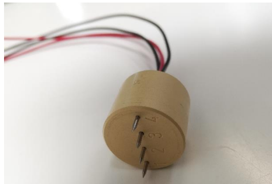
Figure 35: Four needle electrode, with the distance between the needles b = 5.0 mm, radius of the needles r = 0.5 mm and length of the needles L = 5.0 mm
