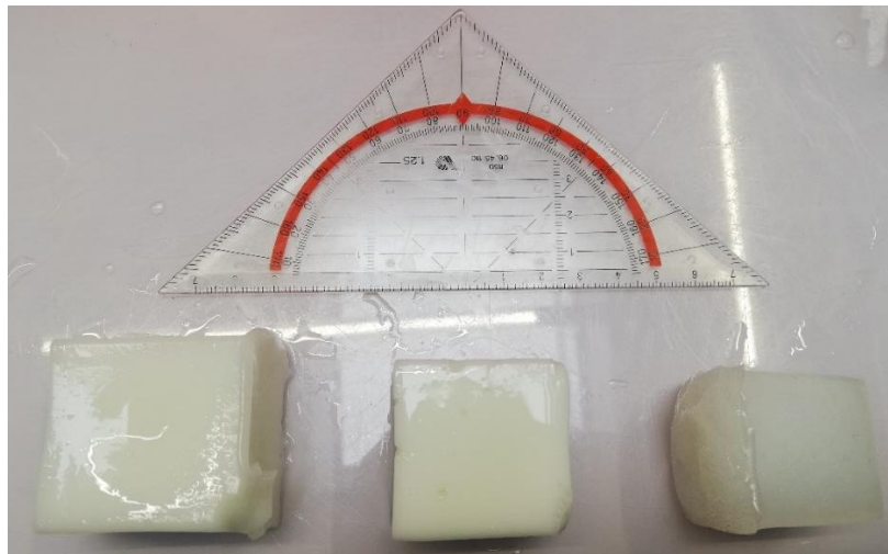
Figure 16: Change in size of PVA-C phantom tissues due to water absorption & drying out of the phantom. Left phantom: stored for 1 week in water. Middle phantom: stored for 1 day in water. Right phantom: stored for 2 days in air.
