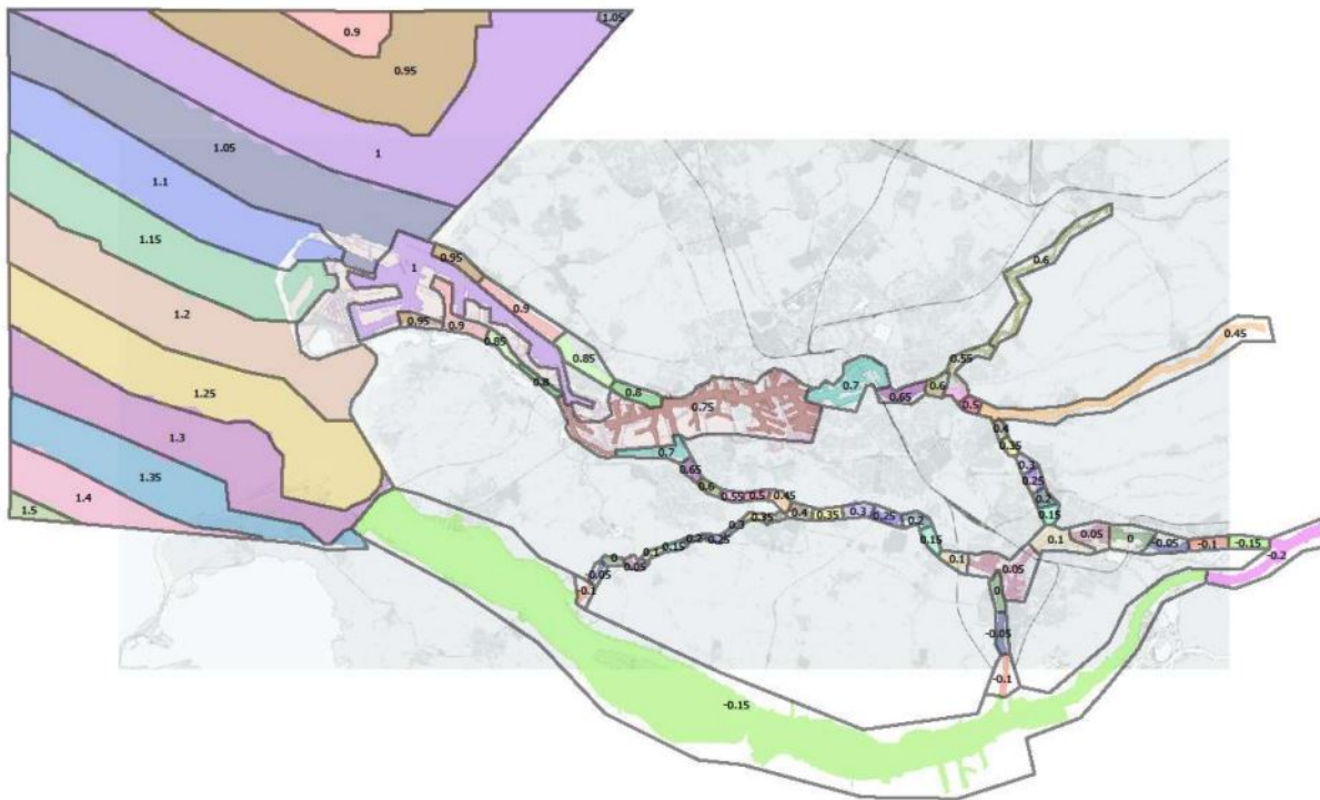
Figure B.1: ALAT regions, where the numbers indicate the height of the NAP reference level with respect to ALAT
