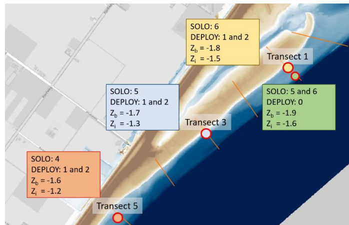
Figure 2.5: Placement of SOLO wave measurement instruments on the PHSD during the HEWO campaign.
