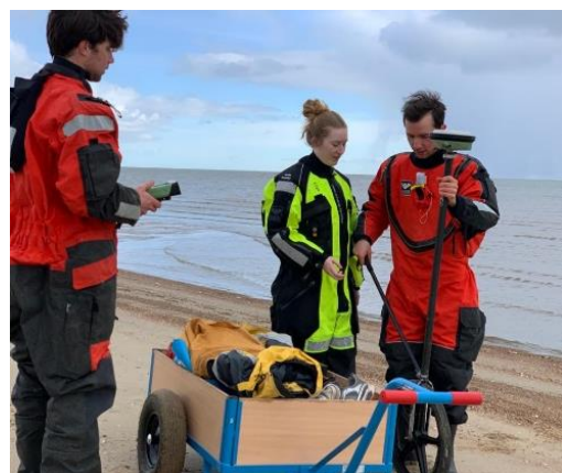
Figure 2.7: Picture of the final field trip on 11 th of March indicating the RTK GNSS GPS measurement set-up with walking wheel and handcart for easy transportation of all equipment over the PHSD.
