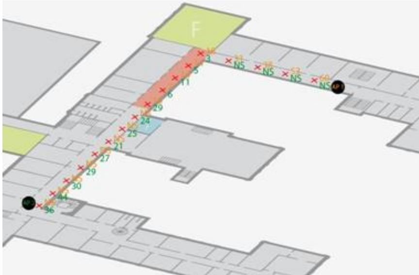
Figure 22: Measured signal strengths of test 3.
