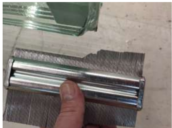
Fig. 5: Measurement of damage using a contour gauge
