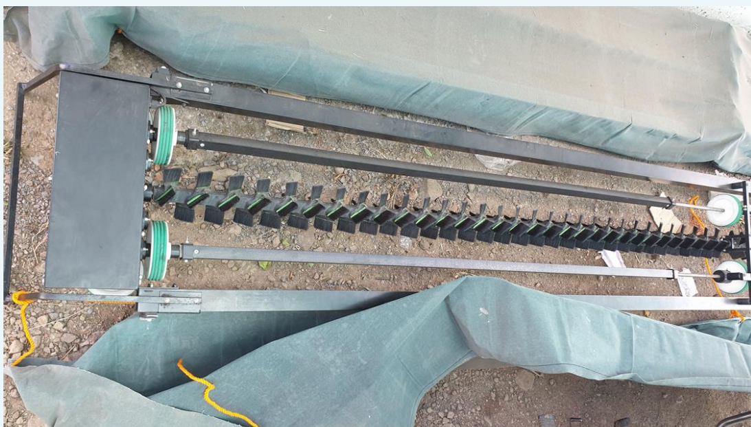
Fig 5.2: Machines brought in to clean the panels (Source: Shamrao)
