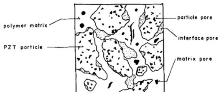
Figure 1.16: Types of porosities in a PZT-polymer composite [43]
