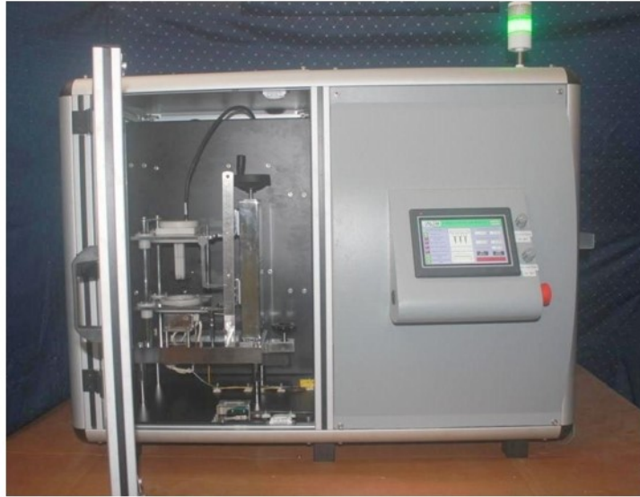
Figure 2.15: Corona poling setup
