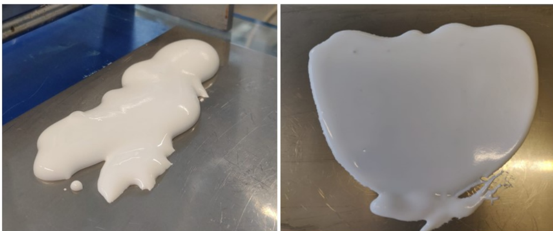
Figure 2.3: Foam before (left) and after (right) tape-casting
