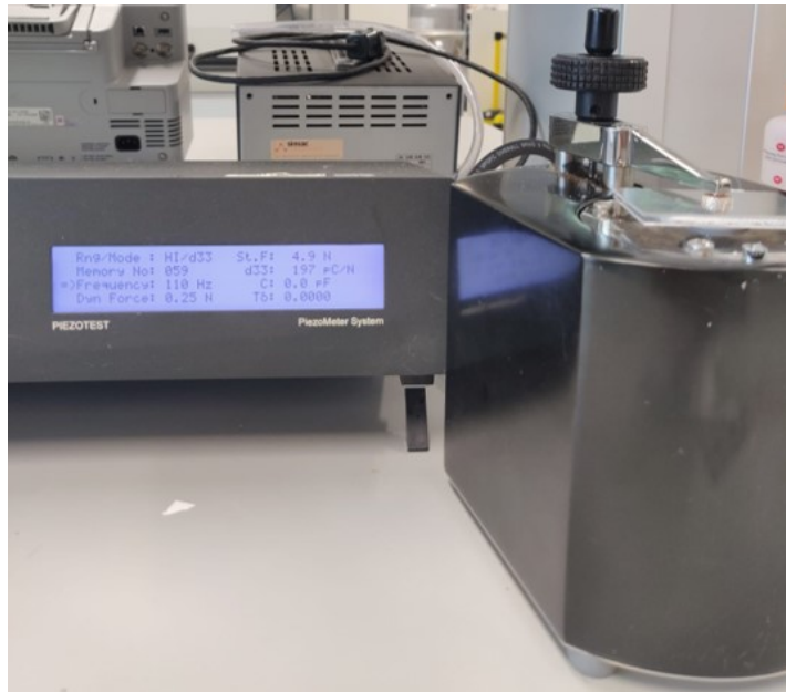
Figure 3.20: Electret behaviour after poling ( d_{33} values in 2 nd column-2 nd row)
