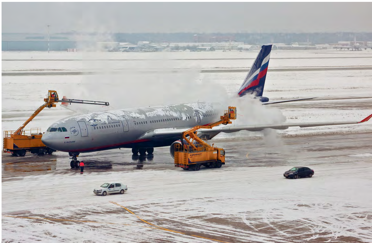
Figure 1.1: De-icing of an airplane with de-icing fluids 1 .
