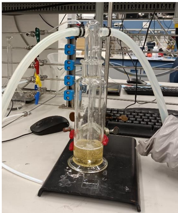
Figure 7 – Gas loading set-up, with the distinct yellow/orange colour of solution showing that it is loaded with \text{CO}_2 .
