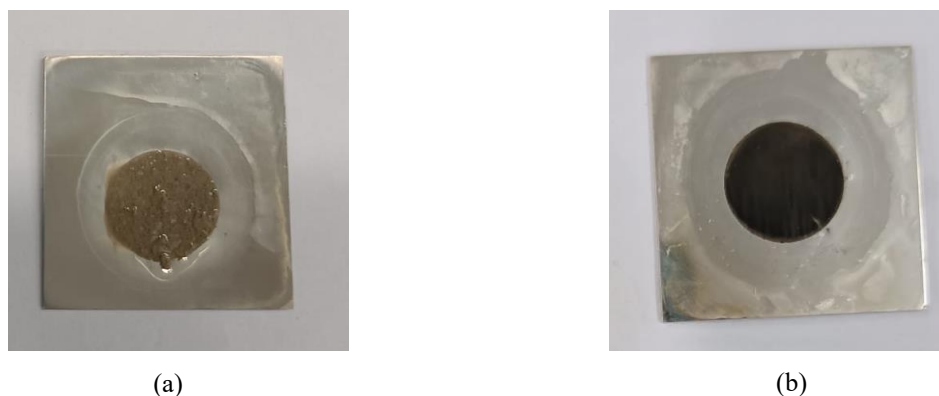
Figure 32 – Comparison of electrodes for (a) -1.5\text{ V} vs. \text{Ag/AgCl} and (b) -1.7\text{ V} vs. \text{Ag/AgCl} of reduction potential with a +0.1\text{ V} vs. \text{Ag/AgCl} 20 second anodic pulse.
