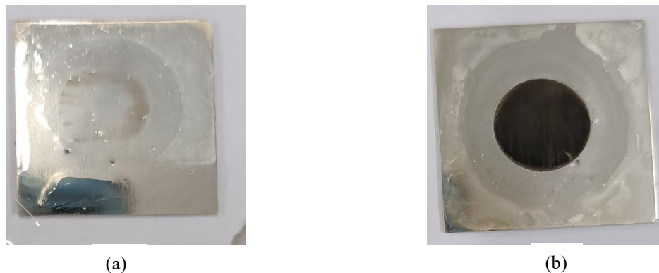
Figure 33 – Comparison of electrodes for (a) -1.7\text{ V vs. Ag/AgCl} (exp. 3) and (b) -1.7\text{ V vs. Ag/AgCl} (exp. 23) of reduction potential with a +0.1\text{ V vs. Ag/AgCl} 20 second anodic pulse.
