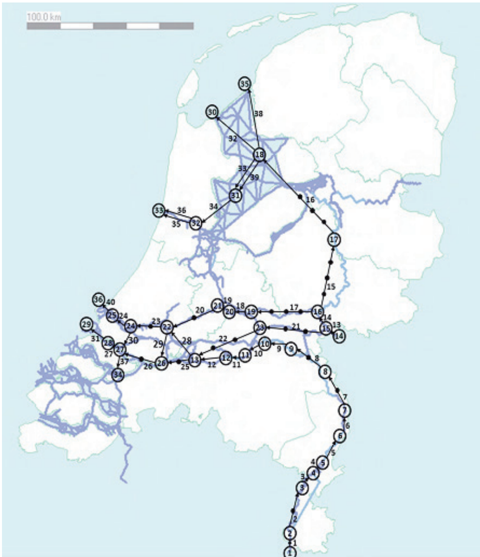
Figure 4-3: Overview of the simplified 1-D hydrodynamic model derived from the SOBEK model (van Overloop, 2011)
