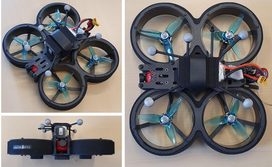
Fig. 2 Top, front and perspective views of the MetalBeetle quadrotor. In these images, the MetalBeetle is shown with the OptiTrack IR marker rig (only used for indoor flights, see section VIII.D) strapped above its battery.
