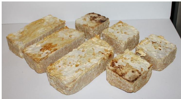
Figure 18. Bricks made in cupboard molds with plastic kitchen foil.
