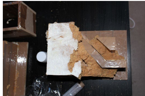
Figure 20. Results of the harvested material of the 9mm MDF molds.
