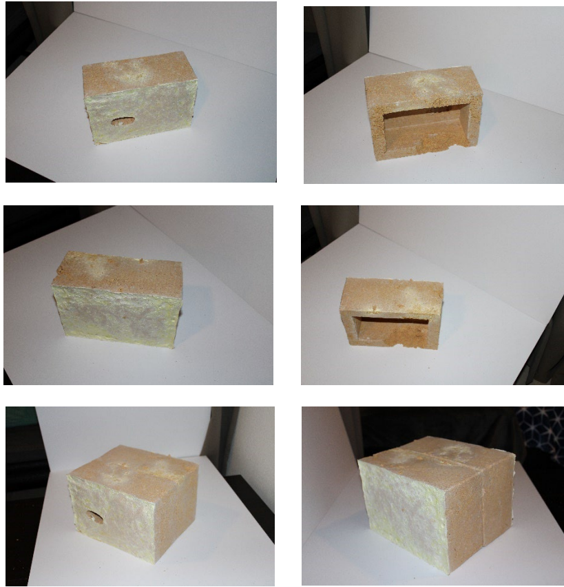
Figure 22. Results of the harvested material of the 6mm MDF molds after completing the whole process.
