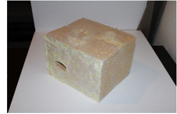
Step 6: Dry the harvested composite for 2 days. Step 7: Bake in 95° Celcius till weighting 35% of its weight. Step 8: The composite is ready.
