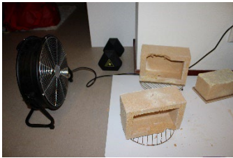
Step 6: Dry the harvested composite for 2 days. Step 7: Bake in 95° Celcius till weighting 35% of its weight. Step 8: The composite is ready.
