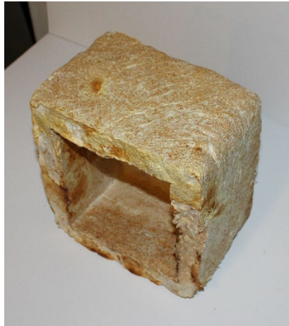
Figure 19. Part of the swift nest box made in cupboard mold with plastic kitchen foil.
