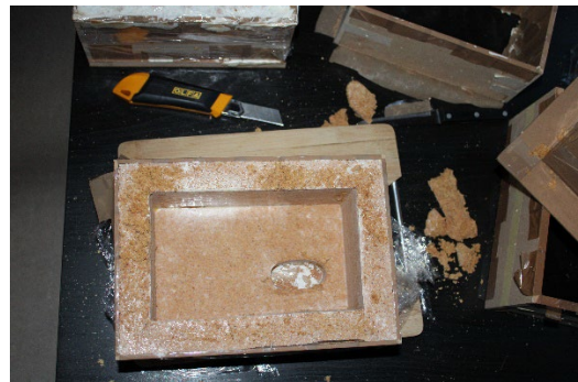
Figure 21. Results of the harvested material of the 6mm MDF molds.
