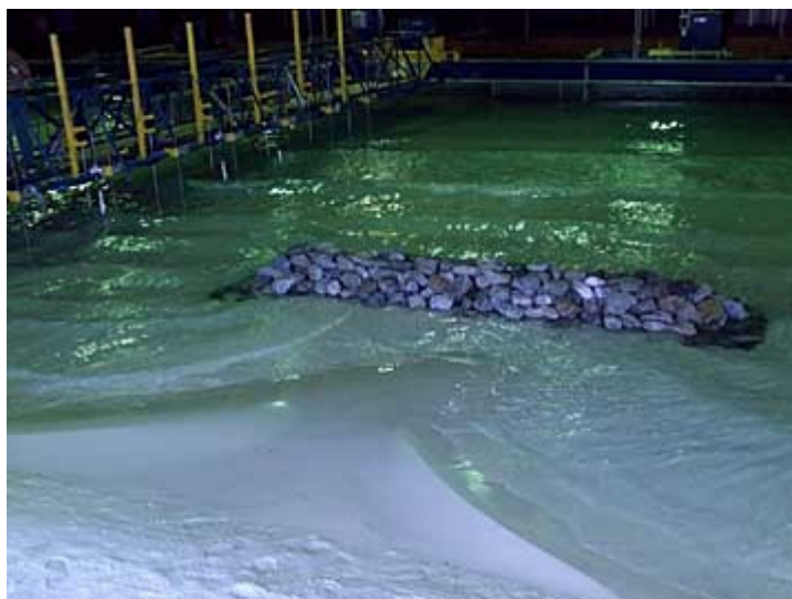
Figure 5.2 A salient behind a detached breakwater
