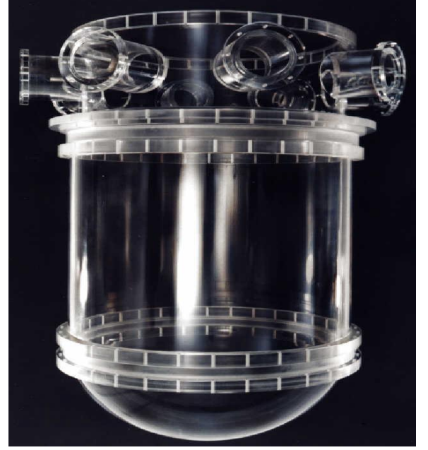
(b) Model of Reactor Pressure Vessel (RPV) at ROCOM facility
