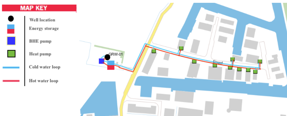
Figure 5-4. The closed loop system connected to a BHE system for the Grouw-01 well.
