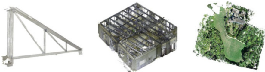
Fig. 3.1 Point clouds at the individual component scale (left: HIR building roof truss, ETH Zurich Hönggerberg Campus), building scale (middle: Kopfbau Halle 118, Winterthur), and landscape scale (right: rehabilitation clinic and grounds, Bettingen)
