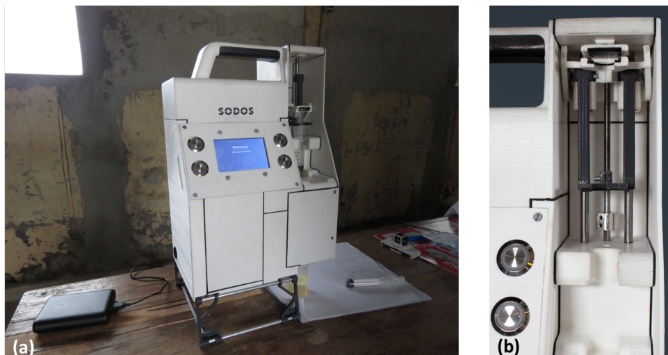
Figure 5. (a) Is the complete diagnostic device and (b) shows the sample injection chamber where the syringe containing 12 ml of infected urine sample is mounted. The urine is pumped through through the micro-channel flow-cell by an attached stepper motor to provide accurate and consistent flow. 1.3 ml of the sample is used to flush out particles from the micro-channel flow cell.
