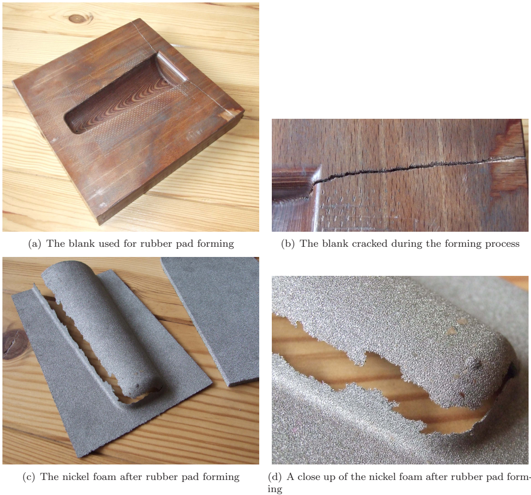
Figure 4.9: Rubber pad forming
