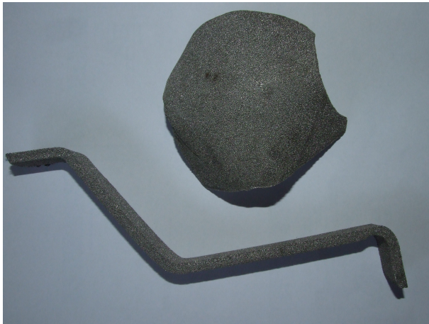
(a) Nickel metal foam after it was shaped around a wooden sphere of 6cm in diameter, the strip has been bend in a sharp edge bending machine
