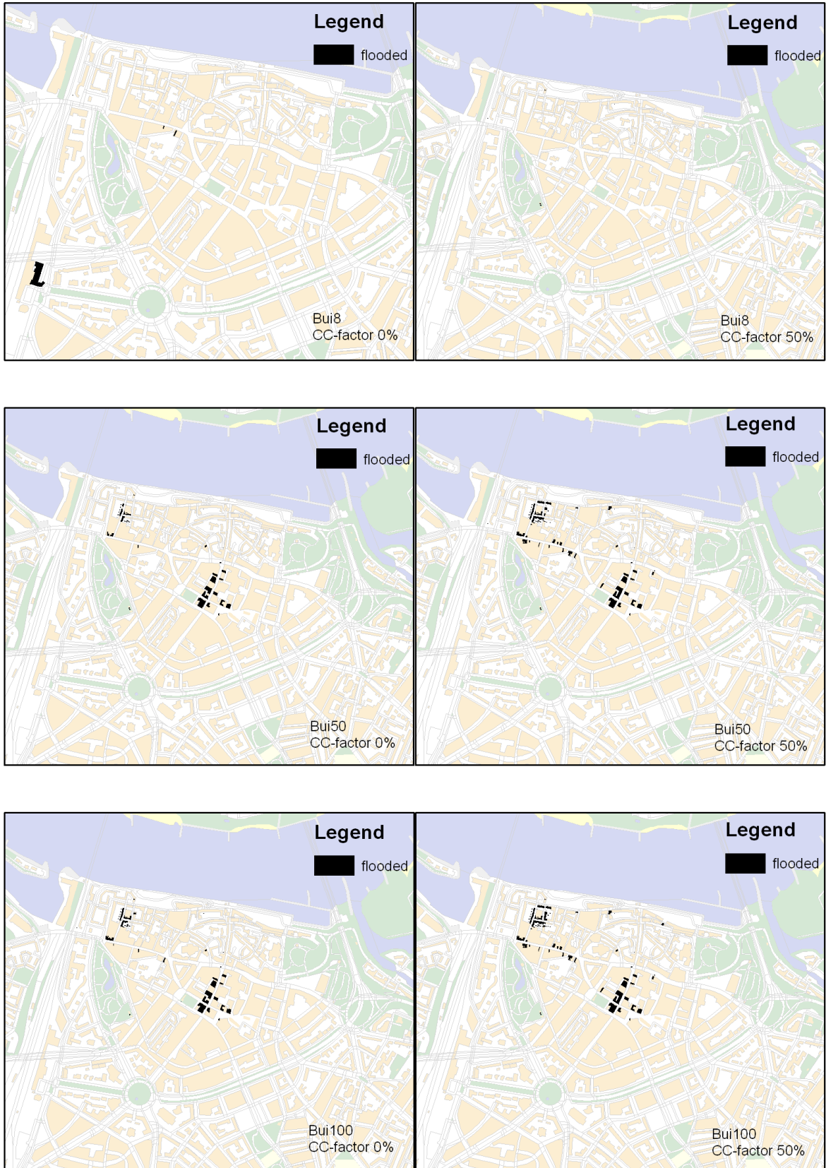
Figure 38 Flooded buildings (assumed doorstep height is 10 cm)
