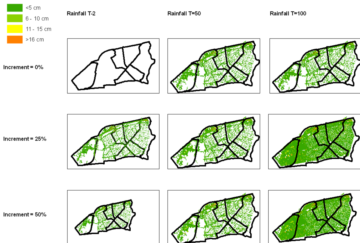
Figure 23 outcomes of the 2D overland flow modelling (T=2, 50 and 100 years and increment=0%, 25% and 50%)
