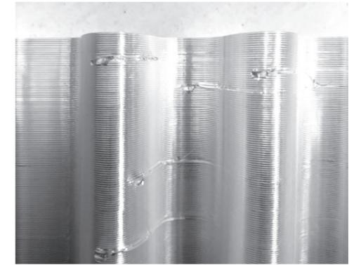
Image: Oozing of layers causing and uneven surface
