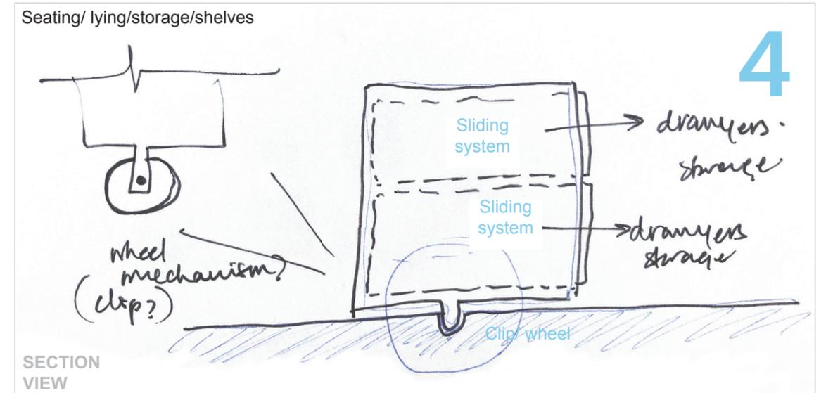
Illustration: Conceptual designs based off functional specifications drawn out from Human Dimensions and interior Spaces (1979) and other functional and conceptual design criteria. These initial conceptual designs will be further developed upon relatively important criteria according to each individual transformable connection, prototyped, tested and validated. (own illustration)
