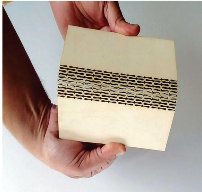
Image: Living hinge template for laser cutting
