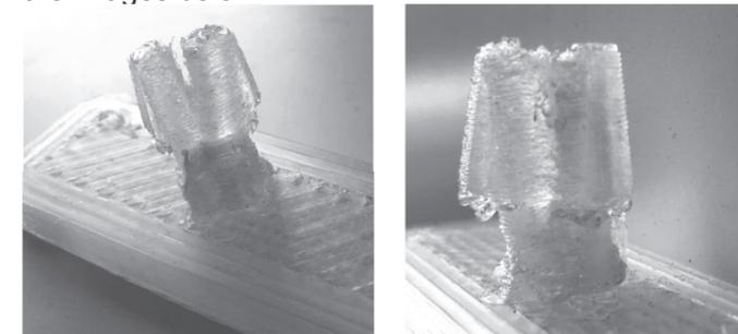
Image: Photographs of prototyped failed clip system (own illustration)
