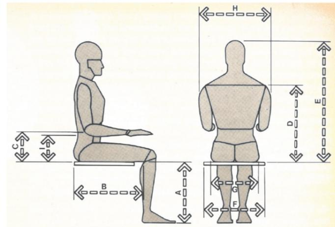
Figure 4-4. Key anthropometric dimensions required for chair design.
