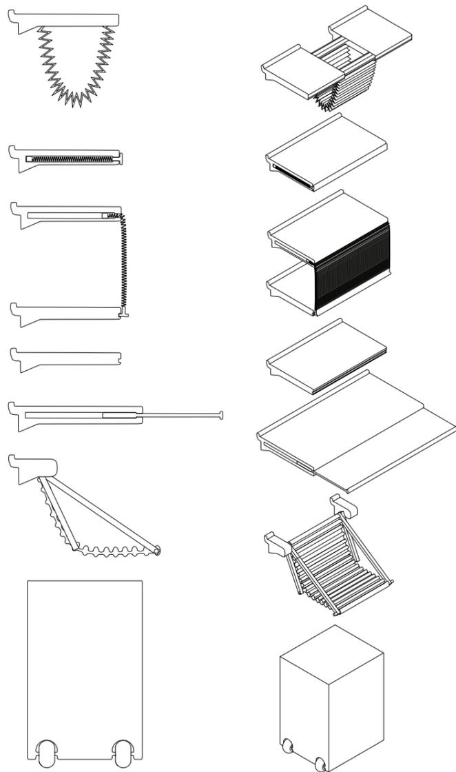
Illustration: section and perspective of designed transformable furniture components (Own Illustration)
