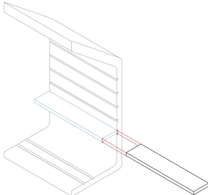
Illustration: Hanging system based on a sliding mechanism (illustrations: own illustration)
