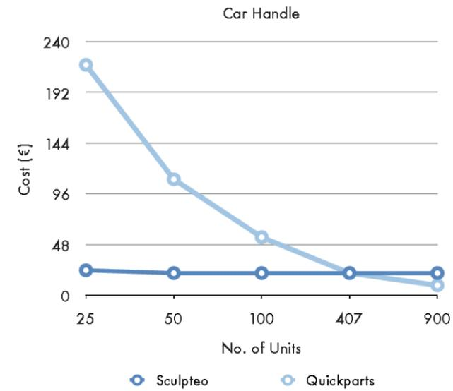
Image: study done by Sculpteo showing the comparative price of a car handle produced by injection moulding (Quickparts) or additive manufacturing. Upto 407 units, it remains cheaper to use 3D printing. Sculpteo.com
