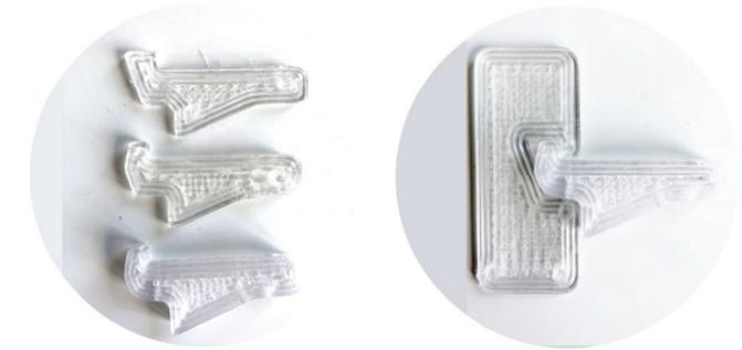
Although the above systems were printed, not every single prototype was a success. As example, the clip system as shown illustrated and photographed, was not a success due to the machinability (oozing of extra material causing the inability to separate the 4 extrusions which would become the slip). This can be seen through the images below.
