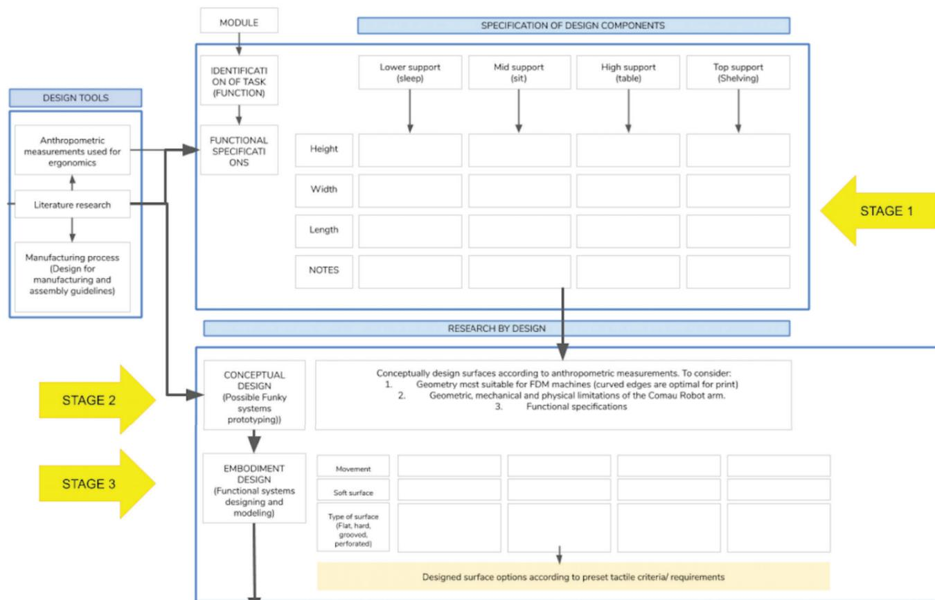
Table 1: Dominant design tools, Stage 1: specification of the design components, Stage 2: conceptual design phase, Stage 3: Embodiment design of the Methodology (own illustration)
