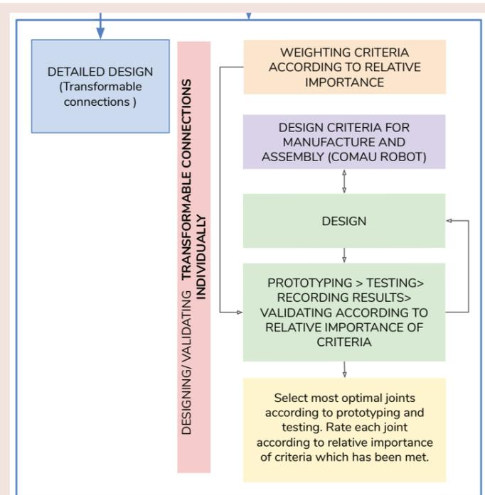
Image: Complete design by research and prototyping cycle for the detailed design phase (Own illustration)
