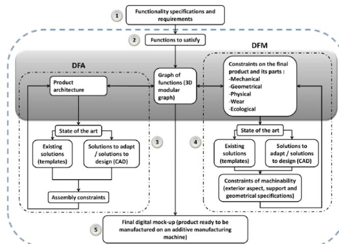
Image: Design methodology for rapid manufacturing (DFRM) (Boyard and Rivette et.al 2013)
