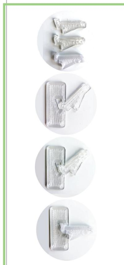
Illustration: Photographs of prototypes printed on a Delta printer using recycled PET as filament (own illustration)
