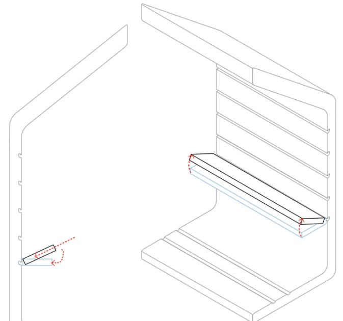
Illustration: Hanging system based on a clip type mechanism (illustrations: own illustration) further used for the development of this transformable connection (own illustration)
