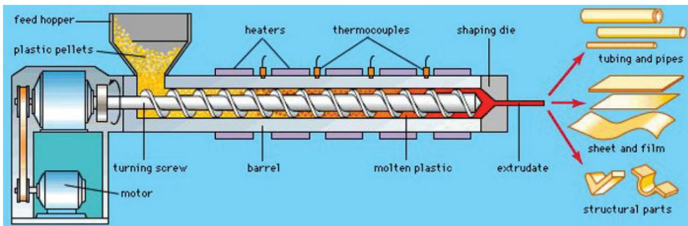
Image: Filament extruder mechanism similar to the one used for the Comau NJ60 2.2
