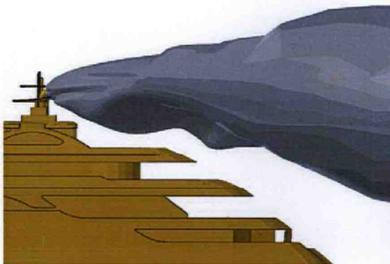
Fig.12: Smoke tracing on fast ferry, Bertram and Couser (2007)
