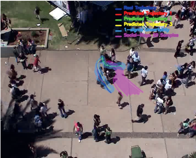
Figure 5.4: Social-VRNN predicted trajectories vs a multi-modal prediction baseline, Social-Ways [93]. In blue is depicted the ground truth trajectory, in red, green and yellow the three possible predicted trajectories by our model, in light blue the one sigma boundary of the predicted trajectory and, in magenta 30 sampled predicted trajectories by the Social-Ways model.
