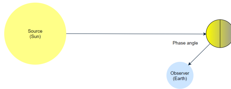
Figure 3.14: Visualization of the phase angle between the source (sun), the observer (earth) and the object. The gradient on the object shows the brightness that is coming from the source. The observer is only able to see part of the sunlit side of the object, causing a drop in perceived brightness.
