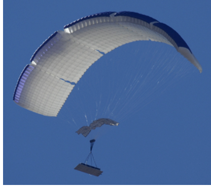
Figure 3.22: Picture of the MegaFly, showing the five different sections of the total surface area
