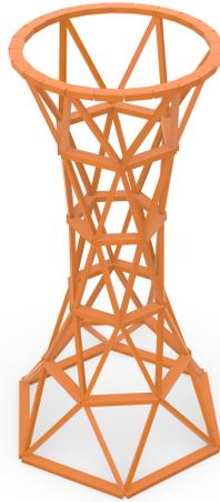
**Figure 8.8:** A sample tower following the triangular topology having segmented rings and a curved ring at the top. This configuration has a shape factor  $N = 6$  and a curvature  $C = -4 m$ .
