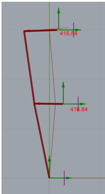
Figure 6.19: Set up of a beam model with curvature  $C = -2.1$   $m$ .
