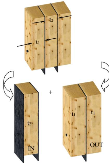
**Figure 8.23:** Decomposition of the connection with four shear planes into connections with two shear planes (Sandhaas et al. 2018).
