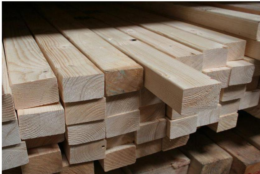
**Figure 2.1:** Sawn timber square elements where knots are visibly present (Woodubuy 2022)
