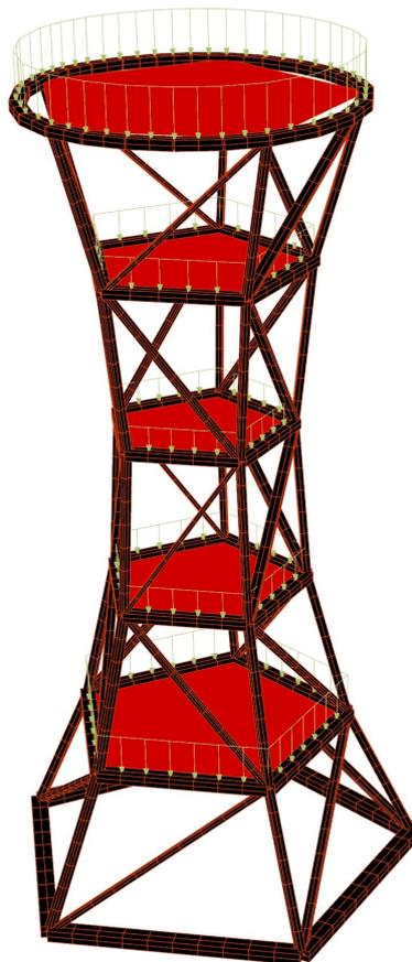
**Figure 8.14:** Applied live and dead loads stemming from a platform at every ring level. Red areas indicate the potential placement of platforms and where live and dead loads are distributed initially.
