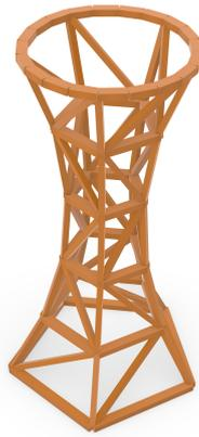
**Figure 8.11:** A sample tower following the custom topology having segmented rings and a curved ring at the top. This configuration has a shape factor  $N = 5$  and a curvature  $C = -4 m$ .
