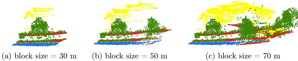
Figure 2.2: Labeled point sets from AHN3, with different block sizes. Ground points are shown in brown, building points are in yellow, water points are in blue and points from others are in green.
