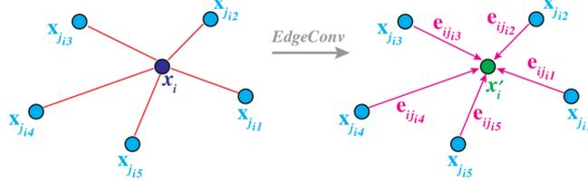
Figure 2.3: The EdgeConv operation [10]. Here the  $k$ -NN graph is constructed with  $k = 5$ . The output  $x'_i$  is calculated by aggregating all edge features associated with the vertex  $x_i$  through a symmetric function (e.g., max pooling).
