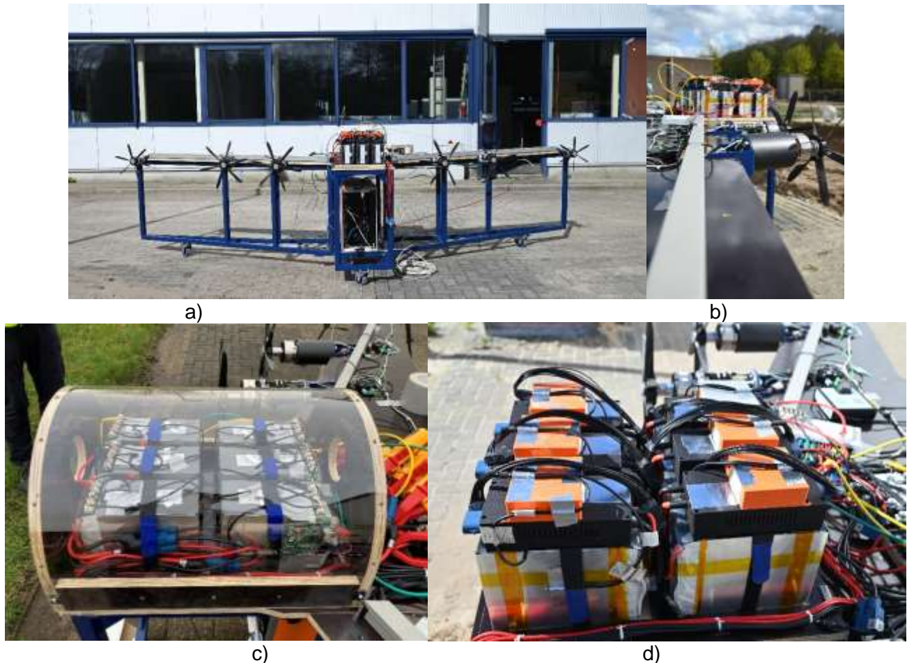
Figure 6 - a) The iron bird, b) the wing of the iron bird with a cable tray mimicking the cable enclosure in the wing, c) the mimic of the fuselage section around the batteries of the iron bird and d) the propulsion batteries with monitoring installed instrumentation on the batteries.
