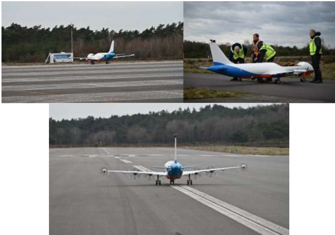
Figure 10 - Pictures of the DEP-SFD during taxi testing at Deelen AFB
