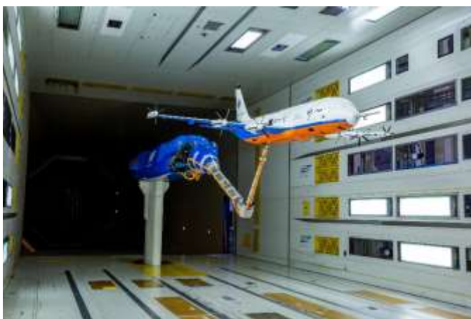
Figure 5 - Scaled aircraft with distributed electric propulsion in the wind tunnel and some results, lift and drag coefficients as a function of flap setting and air speed
