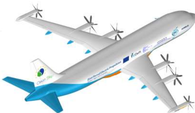
Figure 3 – Computer Aided Design (CAD) model of the DEP-SFD
