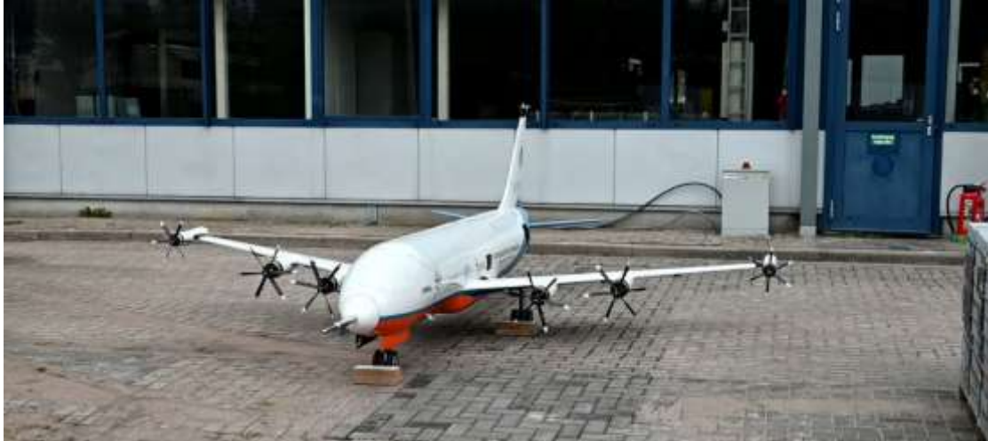
Figure 7 - DEP-SFD installed for stationary ground tests
