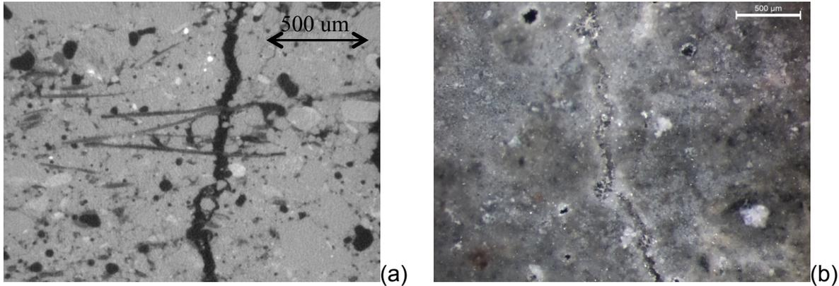
Figure 1: (a) CT image showing Abaca fibres bridging the crack, (b) Crack sealing.
