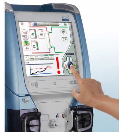
Figure 16: Example of warning system incorporated in a dialysis machine.
