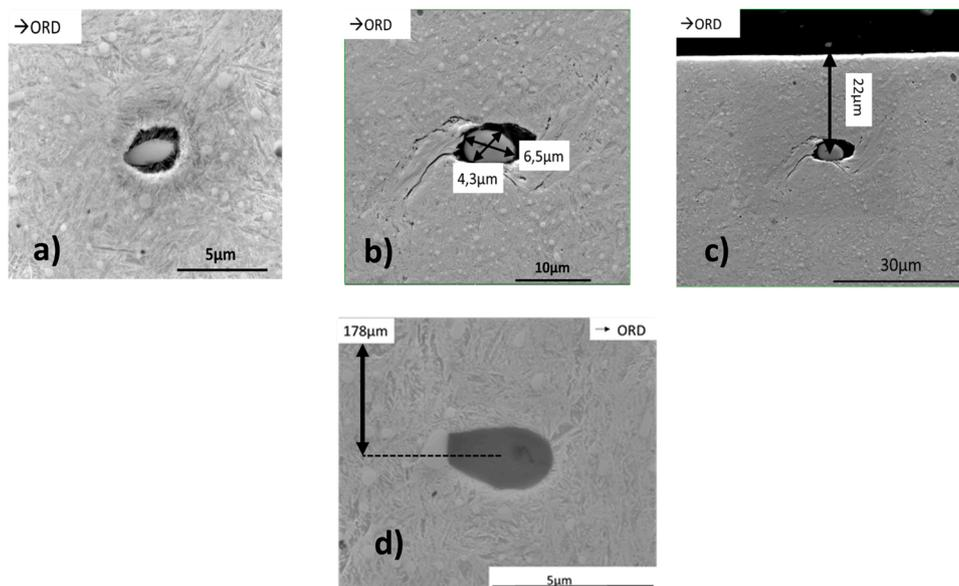
**Fig. 2.** (a) Example of non-metallic inclusion debonded from the matrix, (b) determination of size, and (c) depth below the surface. (d) Fully bonded inclusion, located 178  $\mu\text{m}$  from the raceway surface.
