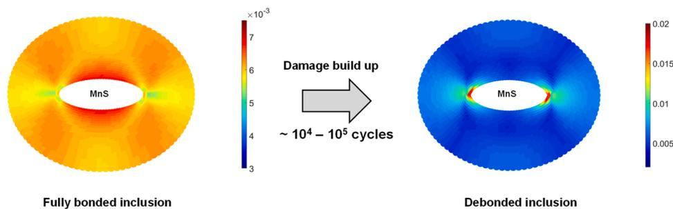
Fig. 12. Crack formation from a NMI via debonding.
