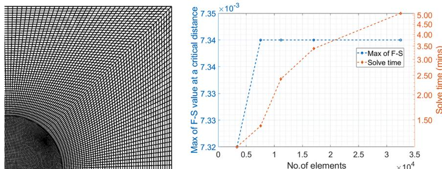
Fig. 5. (a) Mesh design, and (b) mesh convergence.
